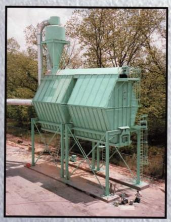
From an Aircon cyclone, many woodworking facilities recycle materials into a bin for truck pickup. This particular application includes valuable safety features such as a spark detection system with multiple abort gates, which is essential in storage areas.
